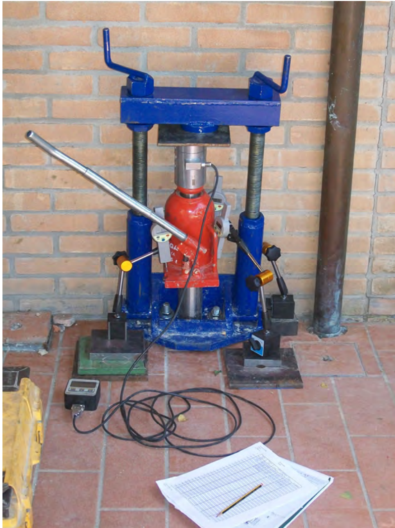
Figure 5: “Castle” apparatus for the execution of compression tests on RR micropiles under an existing foundation.
