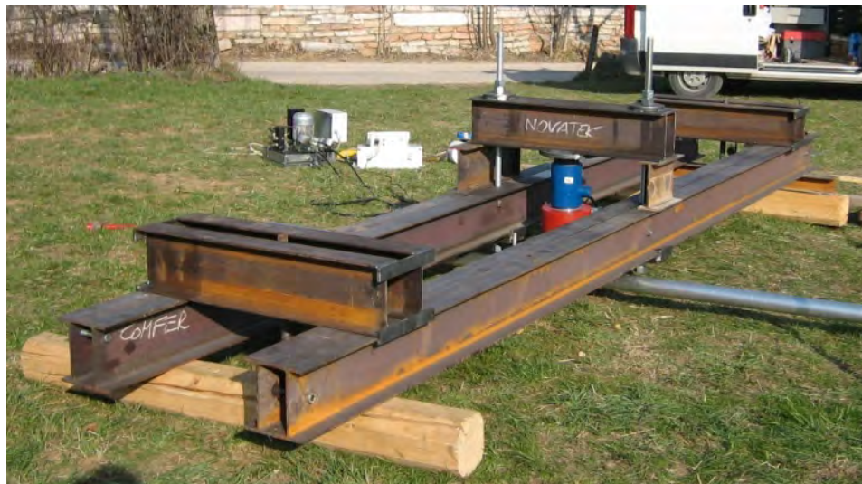
Figure 4: Apparatus with reaction beams for the execution of compression tests at Bosco Chiesanuova (VR).
