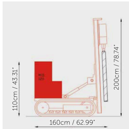
Sectional dimensions of the half-track machine with piling column and opened coring column
